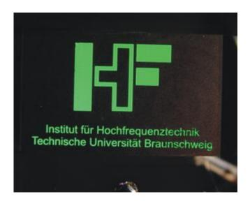
Researchers have designed a simplified OLED that consists of only two organic layers, which here displays the logo of the Technische Universität Braunschweig. At the bottom of the image, two electrical contacts supply the electrical energy. Credit: Meyer, J., et al.
