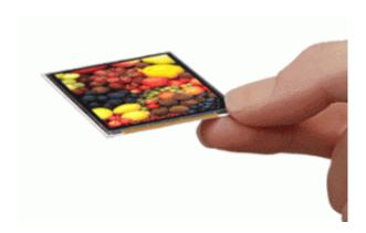
Sharp Corp. has developed a 2.2-inch super-thin LCD for mobile devices with a thickness of only 0.68 mm, the industry's thinnest.
