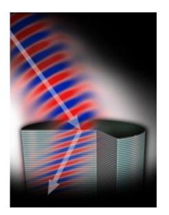
An easy-to-produce material made from the stuff of computer chips has the rare ability to bend light in the opposite direction from all naturally occurring materials. The semiconductors that constitute the Princeton invention are grown from crystals using common manufacturing techniques, making it less complex, more reliable and easier to produce than other metamaterials. Credit: Keith Drake
