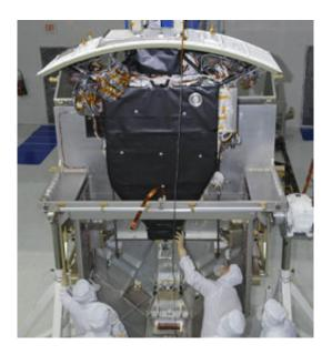
Engineers check NASA's Wide Field Camera 3 instrument to ensure it will fit properly in the protective enclosure that will carry it to orbit aboard the space shuttle next summer for Servicing Mission 4 to the Hubble Space Telescope. Credit: NASA
