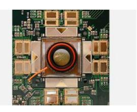
A pinhead size 512-electrode array in the center of this "neuroboard" records the output of retinal neutrons. Credit: Photo by Alan Litke
