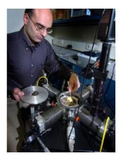
Dimitrios Peroulis, an assistant professor of electrical and computer engineering at Purdue, holds a new MEMS sensor at an "environmentally controlled probe station." The wireless sensors are being developed to detect impending bearing failure in jet engines. The probe station recreates extreme conditions inside engines, enabling researchers to test the sensors. Credit: David Umberger
