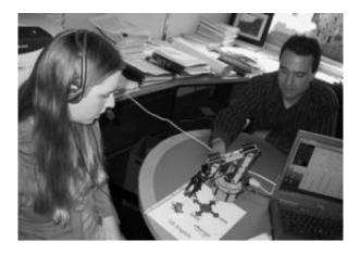
Doctoral student Brandi House uses Vocal Joystick to control the movement of a robotic arm. The screen on the lower right shows how the software analyzes her vocalizations to create instructions for the arm's movement. Credit: University of Washington
