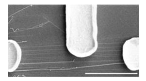
Scanning electron microscope image shows electrodes connected to group of nanowires. Scale bar is five micrometers long. Credit: NIST
