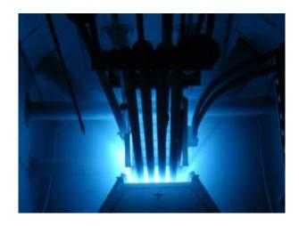
The core of the NCSU PULSTAR reactor at 1-MW power. Credit: NC State University
