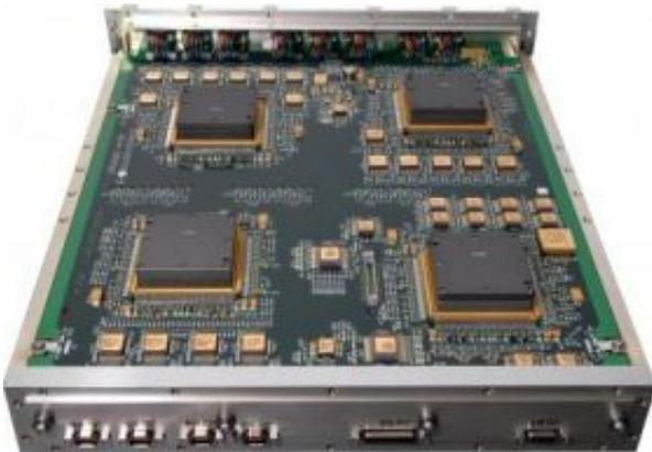
This is the JWST SpaceWire Protocol and Physical Layer Chips on the Multi-SpaceWire Concentrator Card. Credit: NASA
