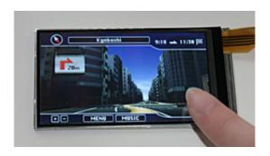
Epson Imaging Devices Corporation today announced the development of an all-in-one liquid-crystal display with an integrated cover (tempered glass or acrylic) and touch panel (resistive or capacitive). This new LCD takes advantage of the company's Photo Fine Vistarich wide viewing angle technology, which enables it to produce beautiful images even when viewed from 90 degrees from the top, bottom, left, or right.
