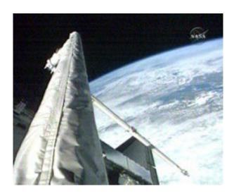
Space shuttle Discovery's robotic arm with the attached boom extension is moved into position shortly after completion of the heat shield inspection. Image credit: NASA
