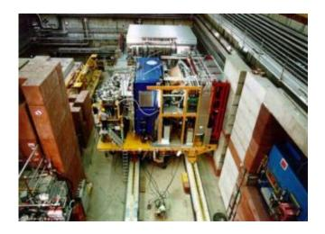
The HERMES experiment (HERA measurement of spin). This photo shows that the entire experiment is mounted on rails and can be moved out of the ring of the particle accelerator (HERA). At the bottom left of the photo a piece of tube from the accelerator can be seen through which the electrons move (to the right).
