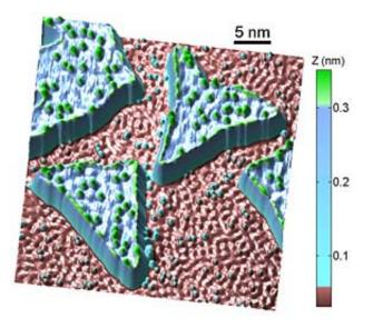
A topographic map of a 4.8 Kelvin (-451°F) copper surface with cobalt islands interspersed. The colors represent height above the copper in nanometers – billionths of a meter. Green specks on the islands are iron "adatoms," while iron adatoms on the copper surface appear blue. The map was obtained with a scanning tunneling microscope with a spin-polarized tip, an instrument that at the same time measured the spin of each iron atom. (Michael Crommie/UC Berkeley)
