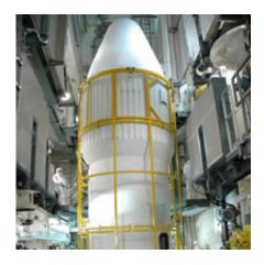
Inside the mobile service tower on Launch Pad 17-B at Cape Canaveral Air Force Station, technicians secure both halves of the fairing around the Dawn spacecraft to the upper stage booster of the Delta II rocket below. The fairing is a molded structure that fits flush with the outside surface of the Delta II upper stage booster and forms an aerodynamically smooth nose cone, protecting the spacecraft during launch and ascent. Image credit: NASA
