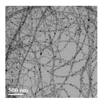
TEM image shows multiwalled carbon nanotubes coated with silver nanocrystals. Credit: Courtesy of Junhong Chen
