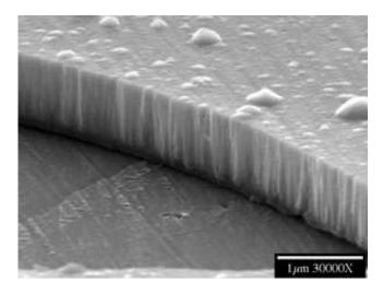
Chemist James Garvey has developed a way to deposit metal oxide onto a polymeric substrate, as shown in this scanning electron microscope image, magnified 30,000 times. Credit: University at Buffalo
