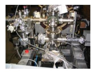
The ultra-high vacuum target chamber, where the intense positron pulse is implanted into the porous silica film. The magnet coils carry a current of 1000 amps for a few hundred milliseconds to generate the strong magnetic field needed to compress the positron beam. Credit: David Cassidy, UC-Riverside
