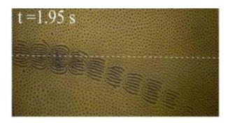
Alternating magnetic fields create snake-like chains of magnetic particles suspended in fluid. The snakes direct the flow of the surrounding fluid along their lengths, potentially leading to new methods to control fluids in chip-based chemical analysis. Credit: M. Belkin, A. Snezhko, I.S. Aranson, and W.-K. Kwok
