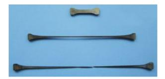
As ductile as a rubber band: Extremely fine and uniformly distributed granules provide new types of steel their "super-plasticity". Above: the original component; middle: symmetrical extension by a factor of 850, below: elongation after fracture at 1025 percent. Image: Max Planck Institute for Iron Research GmbH
