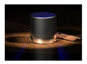
A computer-generated image of the International Prototype Kilogram, which is made from an alloy of platinum and iridium. Image: Wikimedia Commons
