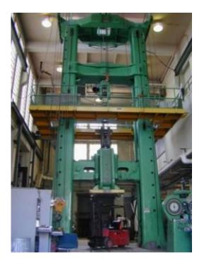
Meet the Baldwin: This 40-foot-tall compression machine is central to the University of Washington's Structural Research Laboratory. The equipment performs full-scale tests for earthquake stresses and extreme loads on ports, buildings and bridges. Soon it will also simulate collapse. Credit: UW
