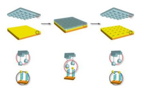
Not-to-scale graphic depicts how catalyst (blue hollow-ended beads) dangles from patterned stamp, while dye particles (gold balls) are bonded to DNA chains to make DNA coating visible. After stamp (blue) presses into DNA coating (yellow) at center the catalyst detaches dye and DNA chain's tip (bottom right). That disruption creates patterning in DNA coating (top right). Graphic by Alexander Shestopalov
