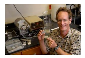
Dr. Steven Bryant, associate professor of petroleum and geosystems engineering, holds two halves of a fractured sample of wellbore cement. Confining the two halves together at pressures similar to those in formations deep below the Earth's surface provides a laboratory model of one type of pathway conceivably allowing carbon dioxide to escape the storage formation. Photo: Erin McCarley
