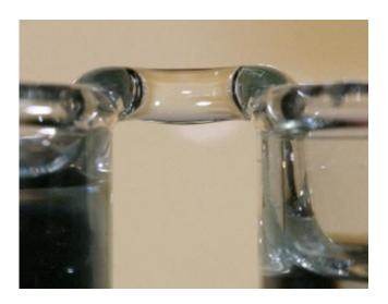
When water in two beakers is exposed to a high voltage, a floating water bridge forms between the beakers. Credit: Elmar Fuchs, et al.
