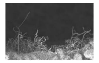
Anodized titanium covered by carbon nanotubes could lead to a new material for orthopedic implants. Credit: Sirinrath Sirivisoot/Brown University
