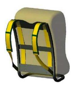
The energy harvesting backpack uses piezoelectric straps to generate electrical energy. Credit: Jonathan Granstrom, et al.
