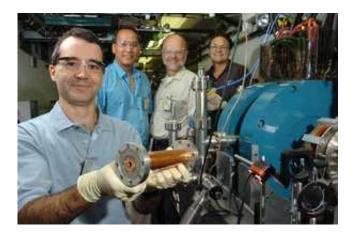
Accelerator physicists Manoel Conde, Zikri Yusof, Richard Konecny and Felipe Franchini stand by the copper-based Argonne Wakefield Accelerator. The wakefield group recently broke the 100 MV/m benchmark for the strength of accelerating gradients by substituting an insulating dielectric for copper.
