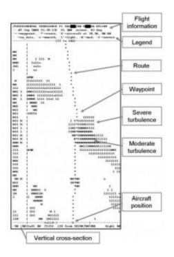
In the cockpit, pilots receive a printout showing areas of turbulence along their flight path. Credit: (Images courtesy Research Applications Laboratory, NCAR)
