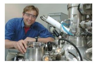
Matthias Bode, Center for Nanoscale Materials, is shown with his enhanced spin polarized scanning tunneling microscope (SP-STM). His enhanced technique allows scientists to observe the magnetism of single atoms. Use of this method could lead to better magnetic storage devices for computers and other electronics. Credit: DOE/Argonne National Laboratory
