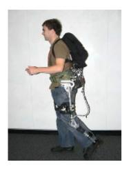
Graduate student Conor Walsh demonstrates a prototype of the 'exoskeleton' he and other MIT researchers have devised. The invention can successfully take on 80 percent of an 80-pound load carried on a person's back. Photo: Samuel Au
