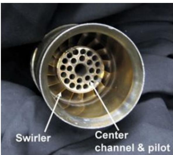
A prototype of the low-swirl injector. Fuel flows through the openings of the center channel. This simple design creates the low-swirl flow, with lower emissions of NO<sub>x</sub> the result. Credit: Berkeley Lab
