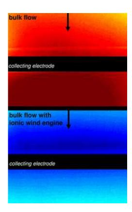
These two infrared images show the cooling effect of an experimental device that uses small "ionic wind engines" developed at Purdue. The red image shows the hot surface of a mock computer chip heated to about 60 degrees Celsius (140 Fahrenheit), and the blue image demonstrates that the device was able to cool the surface to about 35 degrees Celsius (95 F). (Birck Nanotechnology Center image)
