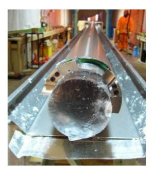
The Dome Fuji deep ice core, Antarctica, with drill. This ice was retrieved from a depth of 1,332 meters (4,370 feet), which was deposited about 89,000 years ago. Photo: Dr. Hideaki Motoyama, National Institute of Polar Research, Japan
