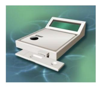
Researchers at PNNL are developing a portable biomonitor to rapidly evaluate tiny samples of blood or saliva for exposure to nerve agents. Credit: Pacific Northwest National Laboratory
