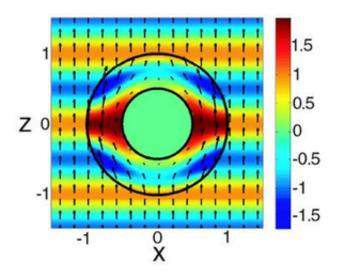
When a polarized plane wave is incident upon an ideal spherical cloak, the object behind the cloak is completely hidden, as shown in this figure (wave arrows from behind pass through the cloak to appear in front). Credit: Chen, et al. ©2007 PRL.
