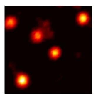
Microscope image of individual fluorescent "polymer dot" nanoparticles spread out on a glass slide. Credit: Jason McNeill, Clemson University
