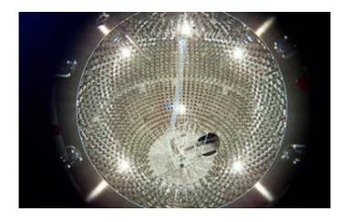
Photomultipliers line the steel chamber of the Borexino detector in this image taken during the detector's construction phase. While the chamber is spherical, the appearance is exaggerated by the distortion of the view through the camera lens. Credit: Virginia Tech; INFN
