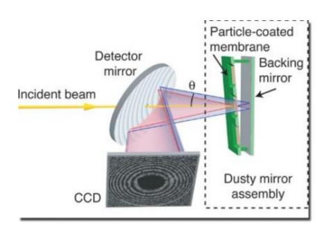
The FEL pulse from the left passes through a hole in a multilayer-coated detector mirror. The "dusty mirror" consists of particles on a 20-nm-thick silicon nitride membrane backed by a multlayer-coated plane mirror. This returns the direct beam back through the hole in the detector mirror, which reflects the diffracted light onto a CCD detector. The prompt diffraction (blue, the reference wave) and delayed diffraction (red, the object wave) interfere to generate the hologram on the CCD detector.
