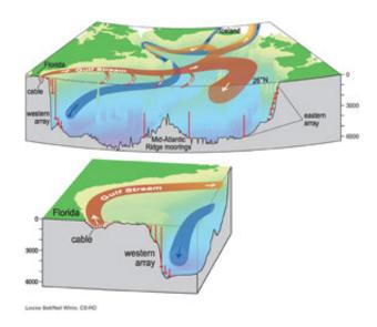
A schematic of ocean currents in the North Atlantic that are now being measured by a network of moored instruments. Image credit – CSIRO
