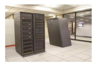
NCAR's BlueGene/L system, code-named "frost," requires a fraction of the power and space of most production systems. The integration of frost brings the capacity of the TeraGrid to more than 250 teraflops of computing capability and more than 30 petabytes of online and archival data storage. Credit: Photo by Carlye Calvin, ©UCAR
