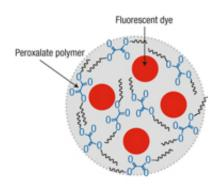
The nanoparticle polymer is made of peroxalate esters. A fluorescent dye (pentacene) is then encapsulated into the polymer. When the nano particles bump into hydrogen peroxide, they excite the dye, which then emits photons (or light) that can be detected. Credit: Georgia Tech
