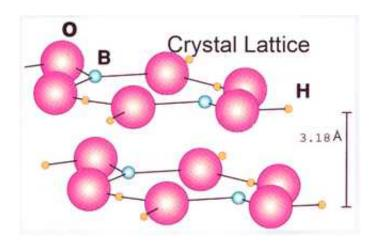
This diagram illustrates the crystalline structure of boric acid. Boron atoms are shown as blue spheres, oxygen pink, and hydrogen brown. Molecular forces that bind the layers in the lattice enable them to slide over one another with very low friction. Credit: ANL
