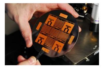
Micro-electromechanical systems (MEMS) are difficult to design, in part because the physics of their tiny moving parts is not fully understood. IMPACT's research will focus on development of CAD systems that are based on physical models and therefore can conclusively predict the behavior of MEMS devices. Georgia Tech Photo: Gary Meek
