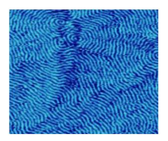
Domain wall pattern for a ferromagnet. The technical use of the magnet is determined by the ease with which the walls can be moved, or equivalently, by the force with which they are pinned. Strong pinning gives a hard magnet, soft pinning a soft magnet. The distance between the walls is 100 nanometers or 10 millionths of a centimeter. Credit: Y-A. Soh and G. Aeppli
