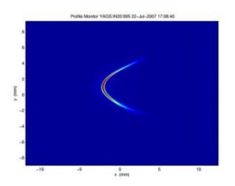
The LCLS electron beam incident on a profile monitor at 135 MeV in the injector spectrometer. This image is taken with the transverse deflecting cavity (LOLA) switched on, producing the curvature, which demonstrates that the beam is accelerated on the crest of the radio frequency wave. Credit: SLAC
