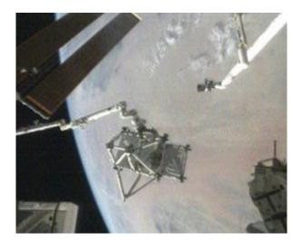
The International Space Station's robotic arm moves the S5 truss. Image: NASA TV
