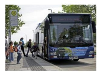
Nuremberg's public transport system has become more "electrified" thanks to a diesel-electric hybrid bus developed by MAN. The vehicle is equipped with drive-system technology from Siemens. The prototype, which also features a special brake energy recovery system, uses up to 25 percent less fuel than conventional buses. The drive system consists of series-produced components, which means mass production of the bus is a possibility that MAN is planning to turn into reality by 2010.
