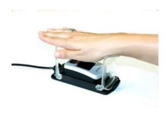
Siemens is expanding its range of biometric access authorization systems to include a hand-surface (palm) reader.
