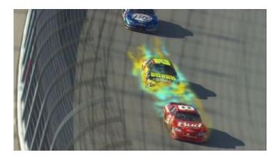
The color of the air indicates the speed and direction of the flow over NASCAR vehicles. ESPN and Sportvision Inc. created the visualization tool, named Draft Track, using an algorithm developed at the UW.
